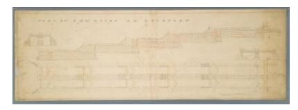
Drawing of locks built on the Erie Canal at Lockport, Niagara County. The locks are drawn in cross-section, seen from above, and seen from the front. The scale is one inch equals eleven feet. The date is unrecorded, but may be ca.1835-1862, during the first enlargement of the canal.
