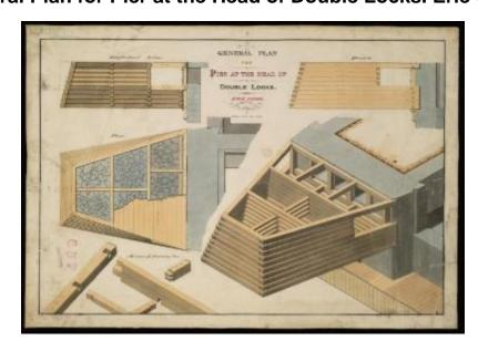
Drawing of a pier to be built at the head of double locks on the Erie Canal. The scale is one inch equals four feet. The date is unrecorded, but may be ca.1835-1862, during the first enlargement of the canal.
