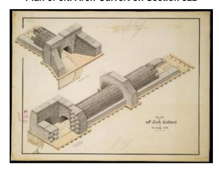
Drawing of an arch culvert to be built in Section 322 of the Erie Canal. The scale is one inch equals four feet. The date is unrecorded, but may be the 1850s as part of the canal's initial enlargement (1835-1862).
