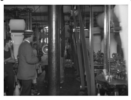
Workmen stand in a room crowded with machinery at the Fulton Street plant of Union Mills, an underwear manufacturer in Hudson, New York. The aisles between machines are very narrow, creating fire and injury hazards. Belts and pulleys on machinery lack protective guards.
