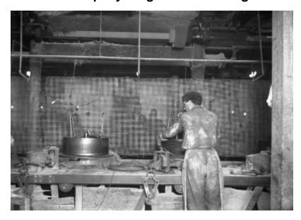
A workman stands at a table guiding wire rope onto a cylindrical drawing machine lacking protective guards at The Waterbury Wire Cable Manufacturing Co. in Brooklyn, New York. One end of the cable trails off the table onto the floor. Behind the work table, a wire or fabric mesh separates this work area from the rest of the room. Silhouettes of other workers are visible through the mesh.
