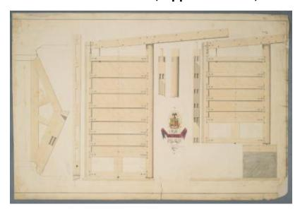
Drawing of gates to be built on a lock of the Erie Canal at "West Troy" (today called Watervliet), Albany County. The scale is three-fourths of an inch equals one foot. The date is unrecorded, but may be ca.1835-1862, during the first enlargement of the Erie Canal.
