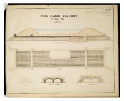
Drawings of a culvert for Fish Creek on the Erie Canal built as part of the canal's first enlargement (1835-1862). No scale is provided. The canal crosses Fish Creek in Ridgeway, Orleans County.
