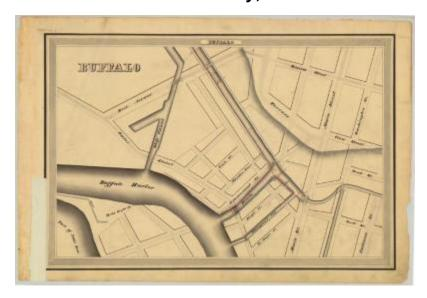
This is an ink, wash and charcoal map of a section of the Erie Canal in Buffalo. It shows part of Lake Erie, Buffalo Harbor, Ship Canal, a canal basin, Thompson's Cut, a guard lock and seven bridges. The red lines indicate courses and distances. The blue lines indicate canal right-of-way. The map also shows seventeen streets in the city of Buffalo.
