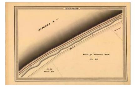
This is an ink, wash and charcoal map of a section of the Erie Canal in Buffalo. It shows The Niagara River, two bridges, two buildings and an unidentified road. The red lines indicate courses and distances. The blue lines indicate canal right-of-way. The map also shows the properties of W. Osborn, Heirs of Frederick Burk and Lot No. 92 and 93.
