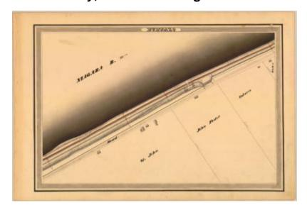
This is an ink, wash and charcoal map of a section of the Erie Canal in Buffalo. It shows The Niagara River, a bridge, nine buildings and an unidentified road. The red lines indicate courses and distances. The blue lines indicate canal right-of-way. The map also shows the properties of St. John, John Foster, Osborn and Walker.
