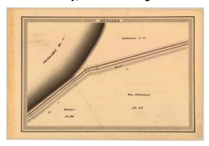
This is an ink, wash and charcoal map of a section of the Erie Canal in Buffalo. It shows The Niagara River, a bridge, four buildings and an unidentified road. The red lines indicate courses and distances. The blue lines indicate canal right-of-way. The map also shows the properties of Walker, Wm. Williams, Williams and Company and Lot No. 94 and 95.
