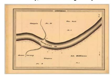
This is an ink, wash and charcoal map of a section of the Erie Canal in Buffalo. It shows Tonawanta Creek with two streams branching off of it, a bridge and four buildings. The red lines indicate courses and distances. The blue lines indicate canal right-of-way. The map also shows the properties of Chapin, James Carney, Simpson, Col. Williams, Wm. Scott and Lot No. 5, 6, 7, 8, 9 and 10.
