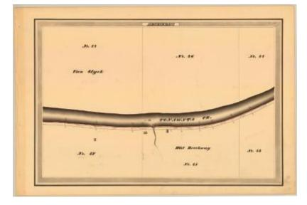
This is an ink, wash and charcoal map of a section of the Erie Canal in Amherst. It shows the Tonawanta Creek, a bridge and three buildings. The red lines indicate courses and distances. The blue lines indicate canal right-of-way. The map also shows the properties of Van Slyck, Hiel Brockway and Lot No. 43, 44, 45, 46, 47 and 48.
