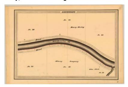
This is an ink, wash and charcoal map of a section of the Erie Canal in Amherst. It shows the Tonawanta Creek, Black Creek, three buildings and two unidentified roads. The red lines indicate courses and distances. The blue lines indicate canal right-of-way. The map also shows the properties of Henry Morley, The Albany Company, John Abbott and Lot No. 21, 22, 23, 24, 25 and 26.
