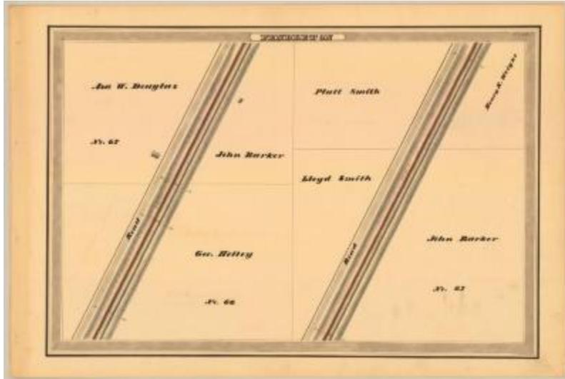
This is an ink, wash and charcoal map of a section of the Erie Canal in Pendleton. The map is split into two views. Both views showing two buildings and an unidentified road. The red lines indicate courses and distances. The blue lines indicate canal right-of-way. The map also shows the properties of Asa W. Douglas, John Barker, Geo. Holley, Platt Smith, Lloyd Smith, Henry K. Wright and Lot No. 66 and 67.
