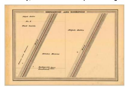
This is an ink, wash and charcoal map of a section of the Erie Canal in Pendleton and Lockport. The map is split into two views. The first view shows the Lockport and Pendleton Town Line, two buildings and an unidentified road. The second view shows a building and an unidentified road. The red lines indicate courses and distances. The blue lines indicate canal right-of-way. The map also shows the properties of Abijah Joslin, Elisha Heacox, Platt Smith, Fellows and Parson and Lot No. 1.
