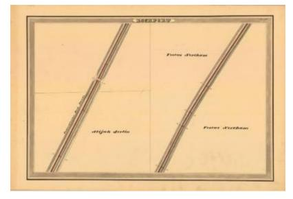
This is an ink, wash and charcoal map of a section of the Erie Canal in Lockport. The map is split into two views. The first view shows rock banks and a bridge. The second view shows only the canal. The red lines indicate courses and distances. The blue lines indicate canal right-of-way. The map also shows the properties of Abijah Joslin and Festus Northam
