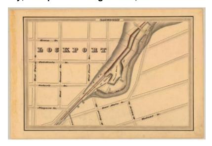
This is an ink, wash and charcoal map of a section of the Erie Canal in Lockport. It shows the City of Lockport, a natural basin, Mill Canal, four bridges and seventeen buildings and mills. The red lines indicate courses and distances. The blue lines indicate canal right-of-way. The map also shows Front Street, Second Street, Third Street, Green Street, Caledonia Street, Ontario Street and Niagara Street.
