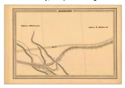
This is an ink, wash and charcoal map of a section of the Erie Canal in Lockport. It shows two buildings and an unidentified road. The red lines indicate courses and distances. The blue lines indicate canal right-of-way. The map also shows the properties of Stephen Wakeman and Oliver L. Millard.
