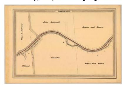
This is an ink, wash and charcoal map of a section of the Erie Canal in Lockport. It shows two buildings, a bridge and an unidentified road, The red lines indicate courses and distances. The blue lines indicate canal right-of-way. The map also shows the properties of Oliver L. Millard, John Griswold, and Rogers and Brown.
