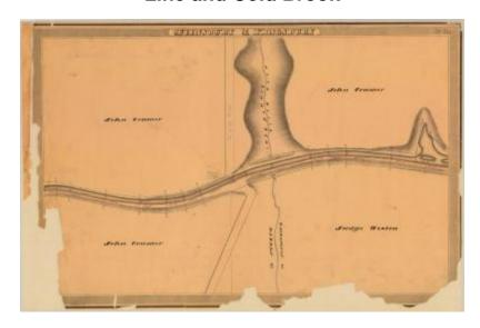
This is an ink, wash and charcoal map of a section of the Champlain Canal Feeder in Queensbury and Kingsbury. It shows Cold Brook which acts as the Warren County and Washington County Line, a triangle shaped basin, a culvert, a bridge and County Line Road. The red lines indicate courses and distances. The blue lines indicate canal right-of-way. The map also shows the properties of John Cramer and Judge Weston.
