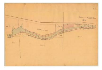
This is an ink, wash and charcoal map of a section of the Champlain Canal Feeder in Queensbury. It shows a large basin, two bridges, three buildings and an unidentified road. The red lines indicate courses and distances. The blue lines indicate canal right-of-way. The map also shows the properties of Walter Geer, Heviland, Langdon and Viely.
