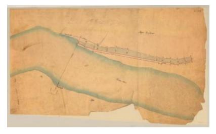
This is an ink, wash and charcoal map of a section of the Champlain Canal Feeder in Queensbury. It shows the Hudson River, the area where the feeder connects to the river, a dock and five buildings. The red lines indicate courses and distances. The blue lines indicate canal right-of-way. The map also shows the property of Roger Heviland.
