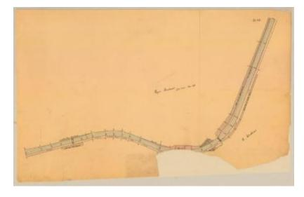
This is an ink, wash and charcoal map of a section of the Champlain Canal Feeder in Queensbury. It shows the feeder and two bridges. The red lines indicate courses and distances. The blue lines indicate canal right-of-way. The map also shows the property of Roger Heviland.
