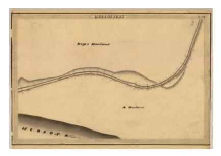
This is an ink, wash and charcoal map of a section of the Champlain Canal Feeder in Queensbury. It shows the Hudson River and two bridges. The red lines indicate courses and distances. The blue lines indicate canal right-of-way. The map also shows the property of Roger Heviland.
