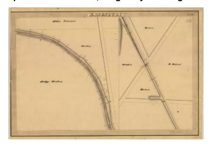
This is an ink, wash and charcoal map of a section of the Champlain Canal Feeder in Queensbury and Kingsbury. The map is split into two views. The first view shows three buildings and an unidentified road. The second view shows a small basin, two bridges and three unidentified roads. The red lines indicate courses and distances. The blue lines indicate canal right-of-way. The map also shows the properties of John Cramer, Judge Weston and B. Baird.
