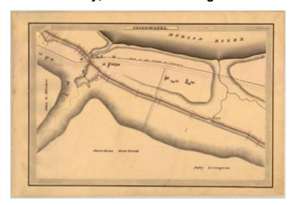
This is an ink, wash and charcoal map of a section of the Champlain Canal in Stillwater. It shows the Hudson River, two waterways running from the river to the canal, two waste weirs, five bridges, twenty-three buildings and the Road to Stillwater Village. The red lines indicate courses and distances. The blue lines indicate canal right-of-way. The map also shows the properties of John Bleeker, Jonathan Rowland and Polly Livingston.
