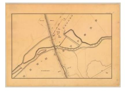
This is an ink, wash and charcoal map of a section of the Chenango Canal in New Hartford. It shows Lock No. 11, the Saquoit Creek which forms multiple streams and channels, a large basin, an aqueduct, a culvert, a bridge and twenty buildings. The red lines indicate courses and distances. The blue lines indicate canal right-of-way. The map also shows the properties of Arnold Mason and E.B. Sherman.
