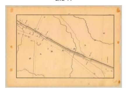
This is an ink, wash and charcoal map of a section of the Chenango Canal in Marshall. It shows Dean's Brook which runs under the canal, Lock No. 42, 43, and 44, a bridge, twenty-two buildings and two unidentified roads that intersect. The red lines indicate courses and distances. The blue lines indicate canal right-of-way. The map also shows the property of William James.
