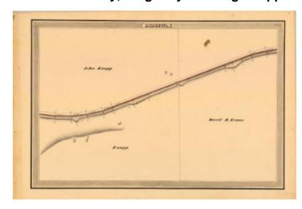
This is an ink, wash and charcoal map of a section of the Erie Canal in Ridgeway. It shows a bridge and six buildings. The red lines indicate courses and distances. The blue lines indicate canal right-of-way. The map also shows the properties of David E. Evans and John Knapp.
