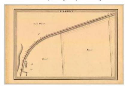
This is an ink, wash and charcoal map of a section of the Erie Canal in Ridgeway. It shows two bridges, three buildings and two unidentified roads. The red lines indicate courses and distances. The blue lines indicate canal right-of-way. The map also shows the property of Isaac Bennet.
