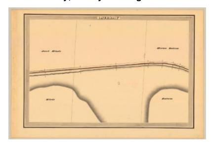
This is an ink, wash and charcoal map of a section of the Erie Canal in Murray. It shows a long straight stretch of the canal that bends slightly and a lone building. The red lines indicate courses and distances. The blue lines indicate canal right-of-way. The map also shows the properties of Jacob Hinds and Horace Balcom.
