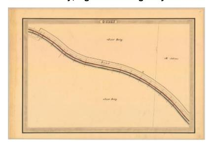
This is an ink, wash and charcoal map of a section of the Erie Canal in Ogden. The map shows a bridge, a building and an unidentified road that crosses the canal. The red lines indicate courses and distances. The blue lines indicate canal right-of-way. The map also shows the properties of Azar Doty and M. Adams.
