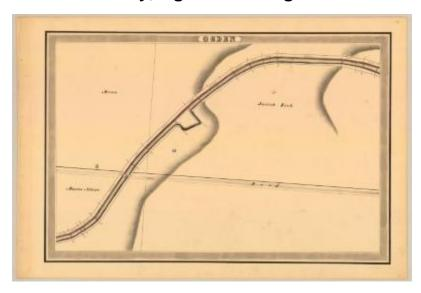
This is an ink, wash and charcoal map of a section of the Erie Canal in Ogden. The map shows a square shaped basin, a bridge, two buildings and an unidentified road that crosses the canal. The red lines indicate courses and distances. The blue lines indicate canal right-of-way. The map also shows the properties of Moon, Josiah Rich and Marcus Adams.
