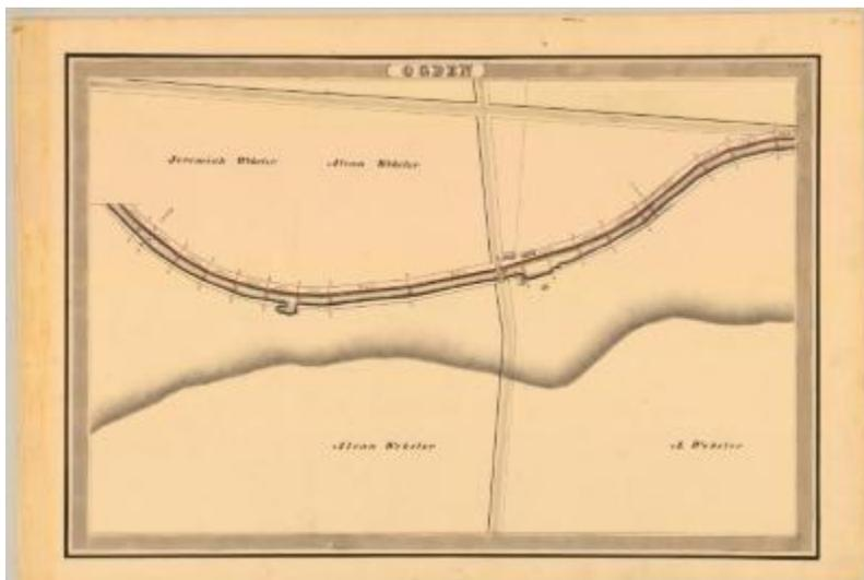
This is an ink, wash and charcoal map of a section of the Erie Canal in Ogden. The map shows a bridge, four buildings and two unidentified roads that intersect. The red lines indicate courses and distances. The blue lines indicate canal right-of-way. The map also shows the properties of Jeremiah Webster and Alvan Webster.
