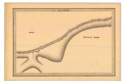
This is an ink, wash and charcoal map of a section of the Erie Canal in Macedon. It shows a small stream that flows into the canal, a building and a portion of a canal bridge. The red lines indicate courses and distances. The blue lines indicate canal right-of-way. The map also shows the property of Barnard Beals and B. Stinson.
