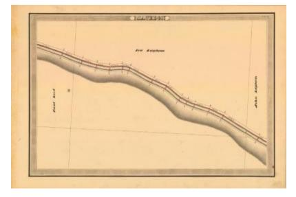
This is an ink, wash and charcoal map of a section of the Erie Canal in Macedon. It shows a stretch of the canal running diagonally across the map and a lone building. The red lines indicate courses and distances. The blue lines indicate canal right-of-way. The map also shows the properties of Paul Reed, Ira Lapham and John Lapham.
