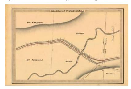
This is an ink, wash and charcoal map of a section of the Erie Canal in Macedon and Palmyra. It shows the Macedon and Palmyra Town Line, Mud Creek which intersects the canal by running under an aqueduct, a bridge, a building and an unidentified road. The red lines indicate courses and distances. The blue lines indicate canal right-of-way. The map also shows the properties of William Chapman, Drake, Joseph Ball and Dr. Robinson.
