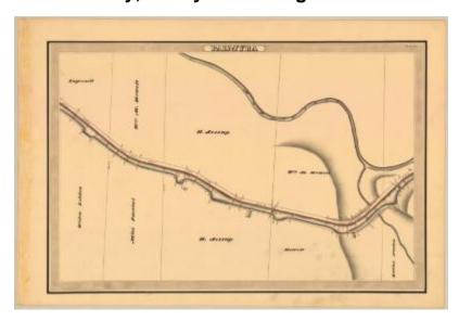
This is an ink, wash and charcoal map of a section of the Erie Canal in Palmyra. It shows the Town of Palmyra, a series of small basins and elongated canal areas, Mud Creek which branches into two streams, two bridges and four buildings. The red lines indicate courses and distances. The blue lines indicate canal right-of-way. The map also shows the properties of Ingersoll, William M. Howell, H. Jessup, Widow Lobdon, Miss Partial and Butler Newton.
