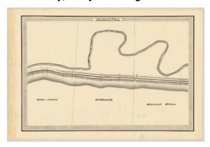
This is an ink, wash and charcoal map of a section of the Erie Canal in Palmyra. It shows Mud Creek which winds along the top of the canal and a small bridge. The red lines indicate courses and distances. The blue lines indicate canal right-of-way. The map also shows the properties of Butler Newton, Goldsmith and Hazard Wilcox.
