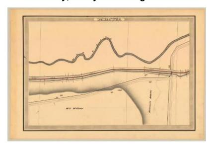
This is an ink, wash and charcoal map of a section of the Erie Canal in Palmyra. It shows Mud Creek which runs along the top of the canal, two bridges, seven buildings and two unidentified roads that meet and cross the canal. The red lines indicate courses and distances. The blue lines indicate canal right-of-way. The map also shows the property of William Wilcox and Francis Bartle.
