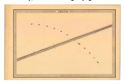
This is an ink, wash and charcoal map of a section of the Erie Canal in Junius. It shows a straight diagonal run of the canal and the Cayuga Marsh. The red lines indicate courses and distances. The blue lines indicate canal right-of-way.
