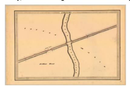
This is an ink, wash and charcoal map of a section of the Erie Canal in Junius. It shows the Cayuga Marsh, the Canandaigua Outlet which runs into the canal, a mud lock, a bridge that spans the outlet and a building. The red lines indicate courses and distances. The blue lines indicate canal right-of-way. The map also shows the property of Jethro Wood.
