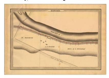
This is an ink, wash and charcoal map of a section of the Erie Canal in Minden. It shows the Mohawk River, two rounded basins, a bridge, six buildings, the Road to Fort Plain and an unidentified road that leads to a rope ferry. The red lines indicate courses and distances. The blue lines indicate canal right-of-way. The map also shows the properties of A.F. Fralick, W. Knieskern and the Heirs of A. Devendorf.
