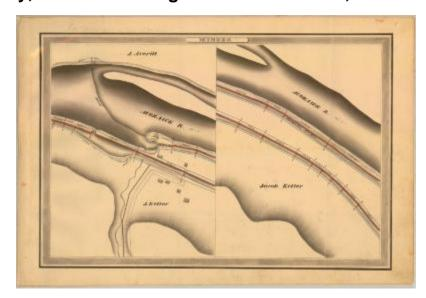
This is an ink, wash and charcoal map of a section of the Erie Canal in Minden. The map is split into two views. The first view shows the Mohawk River, a dam, a guard lock, a bridge, seven buildings including a saw mill and an unidentified road. The second view shows the Mohawk River and a navigable feeder. The red lines indicate courses and distances. The blue lines indicate canal right-of-way. The map also shows the properties of J. Averill and Jacob Keller.
