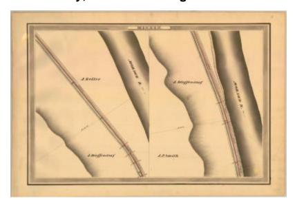
This is an ink, wash and charcoal map of a section of the Erie Canal in Minden. The map is split into two views. Both views show the Mohawk River and the canal. The red lines indicate courses and distances. The blue lines indicate canal right-of-way. The map also shows the properties of Jacob Keller, J.P. Smith and J. Dieffendorf.
