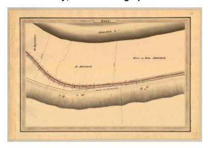
This is an ink, wash and charcoal map of a section of the Erie Canal in Root. It shows the Mohawk River, two bridges, seven buildings and the Road to Fultonville. The red lines indicate courses and distances. The blue lines indicate canal right-of-way. The map also shows the properties of G. Spraker, H. Mitchell and the Heirs of William Mitchell.
