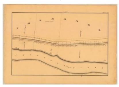
This is an ink, wash and charcoal map of a section of the Chenango Canal in Chenango. It shows the Chenango River which runs along the bottom of the canal, four buildings and an unidentified road. The red lines indicate courses and distances. The blue lines indicate canal right-of-way. The map also shows the properties of Joseph J. Terwilleger, Diodate Cushman and Christopher Eldredge.
