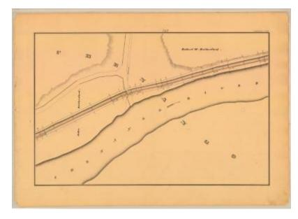
This is an ink, wash and charcoal map of a section of the Chenango Canal in Chenango. It shows the Chenango River which runs along the bottom of the canal, a bridge and two unidentified roads. One of these roads crosses the canal. The red lines indicate courses and distances. The blue lines indicate canal right-of-way. The map also shows the properties of John Rutherford and Robert W. Rutherford.
