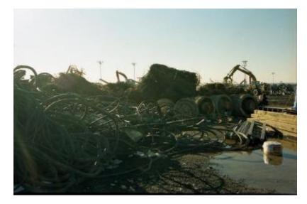
Cables on left, five WTC elevator motors on ground (with orange paint) and WTC rebar in rear.
